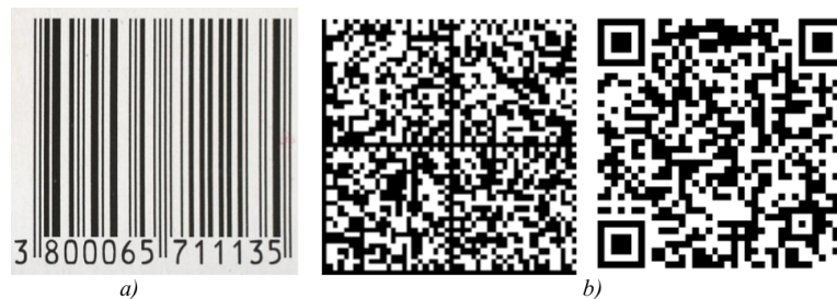
Figure 1.15: Engraving of bar-codes: a) 1D; b) 2D [51, 52].
