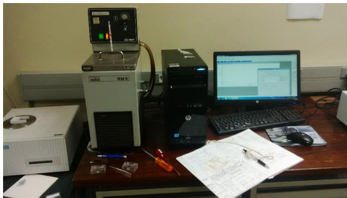
Image 8. Perkin-Elmer Pyris 6 Thermogravimetric analyzer.
