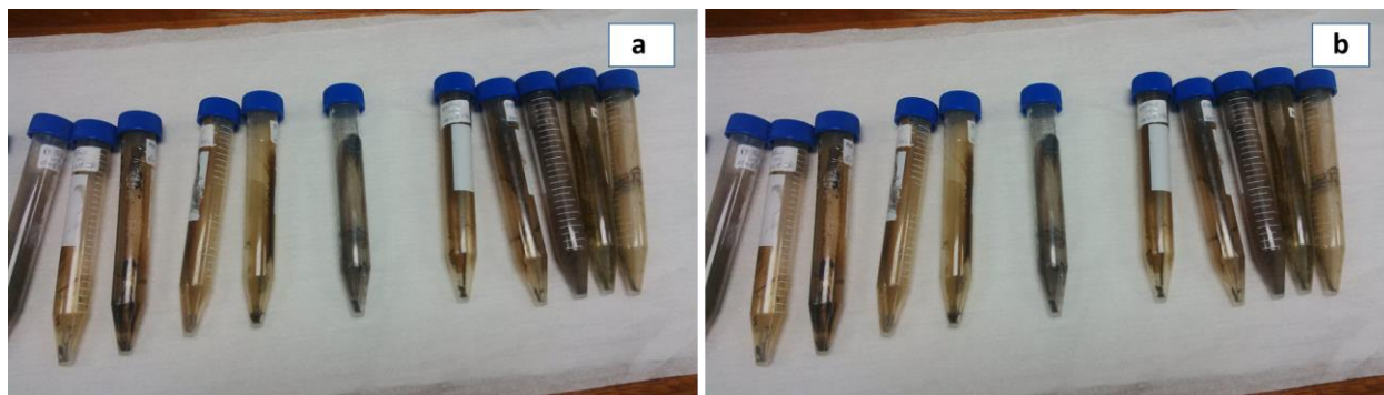
Image 2. Some tubes of synthesized a) DT-capped \text{Cu}_x\text{S}_y and b) OLA-capped \text{Cu}_x\text{S}_y nanoparticles.
