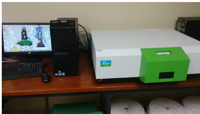
Image 13. Perkin-Elmer LS 55 spectrofluorimeter.
