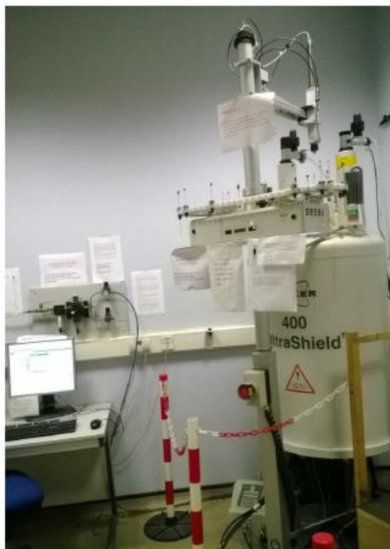
Image 10. Nuclear magnetic resonance Bruker advance III 400 MHz spectrophotometer.
