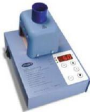
Image 6. Barloworld SMP10 Melting Point Apparatus.
