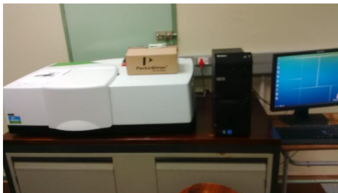
Image 11. Perkin Elmer Lambda 1050 UV/Vis/NIR spectrophotometer.
