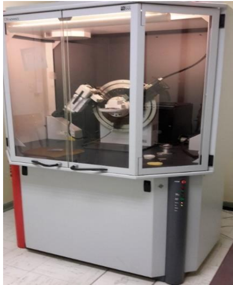
Figure 26. Bruker AXS D8 Advanced X-ray diffractometer (UZ, SA).
