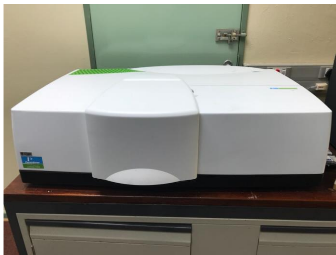
Figure 20. Perkin Elmer Lambda 1050 Near IR UV/Visible spectrometer (UZ, SA).
