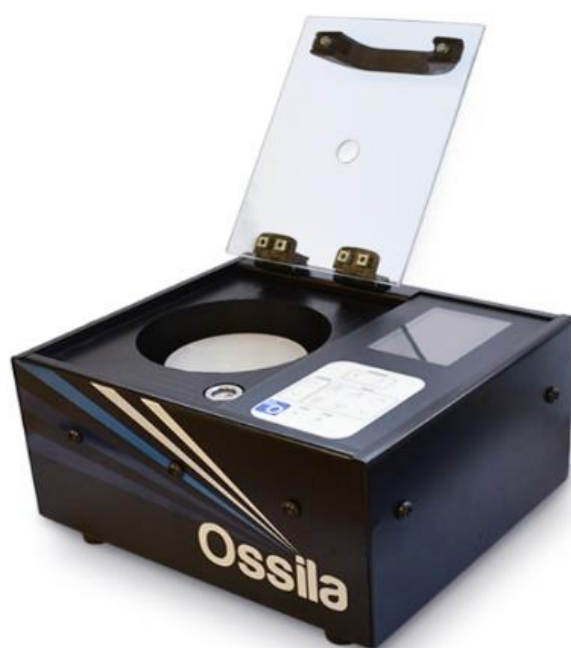
Figure 18. Ossilla Spin Coater (UZ, SA).
