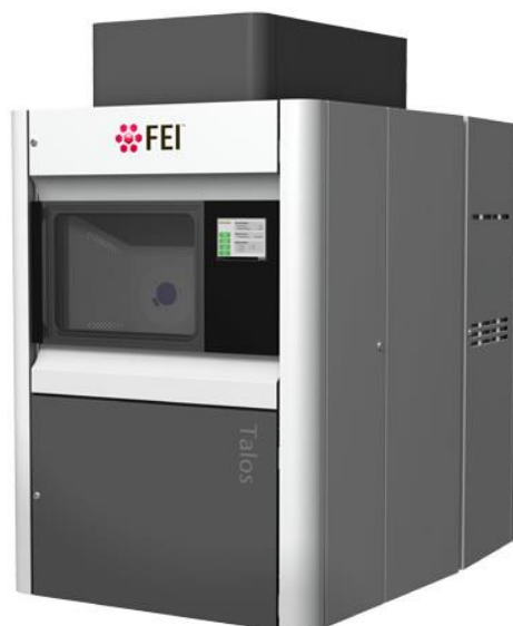
Figure 23. FEI Talos F200A HRTEM microscope (TUM, UK).
