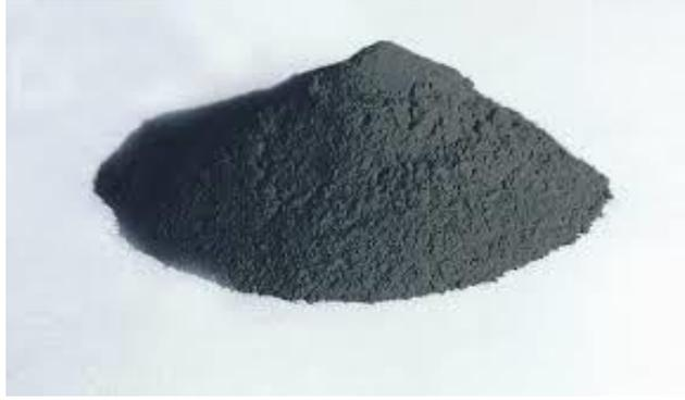
**Figure 7: Powder activated carbon**
