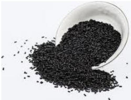
**Figure 8: Granular activated carbon**
