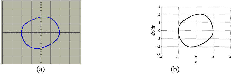
Figure 3.2 Phase portrait exhibited by one oscillator before the coupling: (a) Experiment and (b) Numerical.
