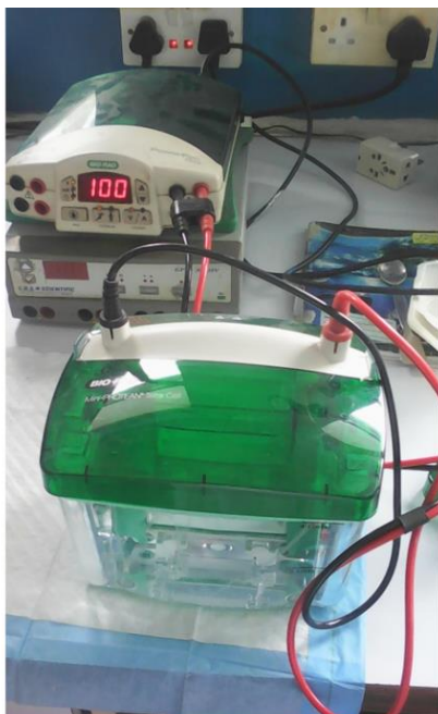
Figure 32: Montage de SDS-PAGE
