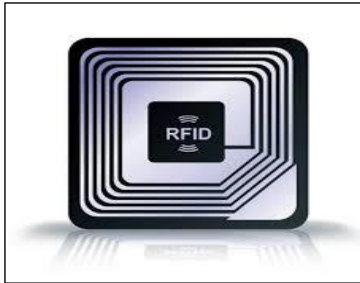
Figure II.15 : étiquette RFID passive [18]
