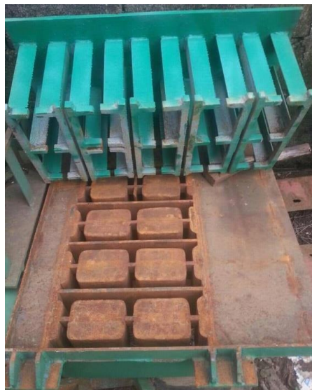
Figure 11: moule de parpaing traditionnel [6]
