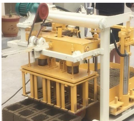
Figure 12: pondeuse semi -automatique [8]
