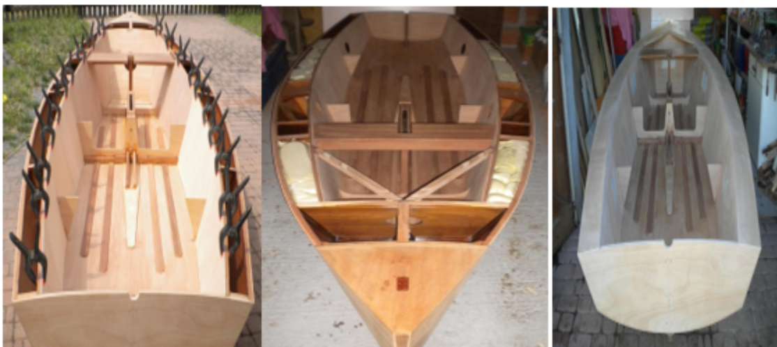
FIGURE 3.9 – Caissonage du bateau
