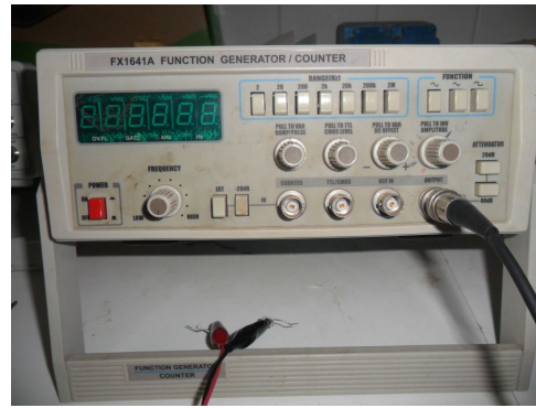
(b) FX1641A, Function generator counter, 2 MHz
