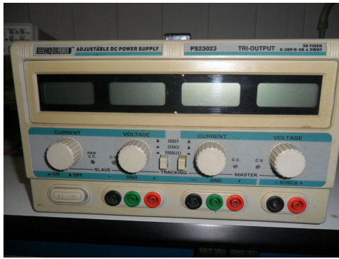
(a) PS2303, Tri output 5 V fixed, 0 – 30 V/0 – 3 A × 2 ways
