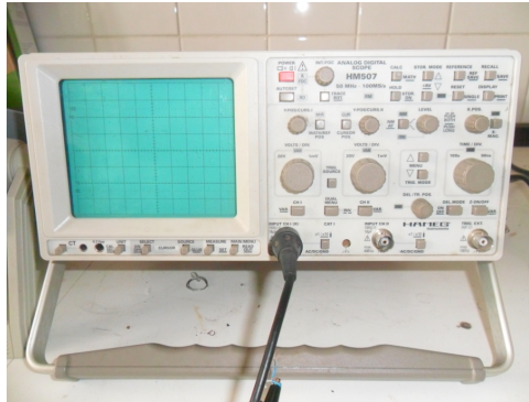
(c) HM507, Digital oscilloscope, bandwidth 0 – 50 MHz, rise time < 7 ns
