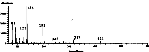
Figure 4. EI spectrum of trifluoroacetylated \alpha -terpineyl 6- O -( \alpha -L-arabinofuranosyl)- \beta -D-glucopyranoside (tentatively identified).
