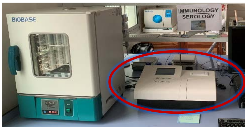
ELISA reader used to measure absorbance in samples at the end of experiments
