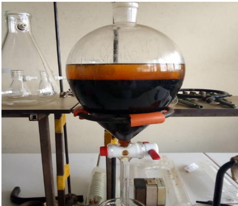
Figure 23: Extraction liquide-liquide de Hunteria ballayi
