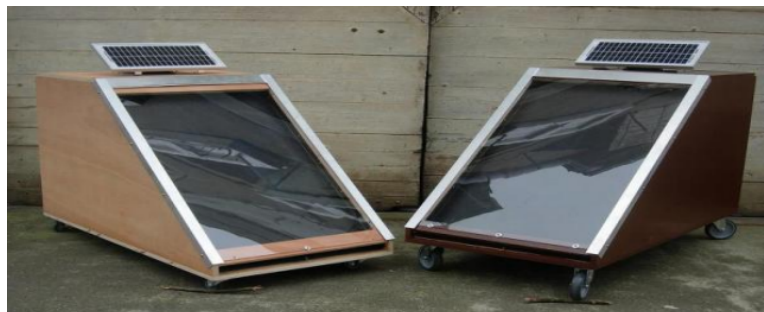
FIGURE 1.13 – SSéchoir solaire hybride [37]
