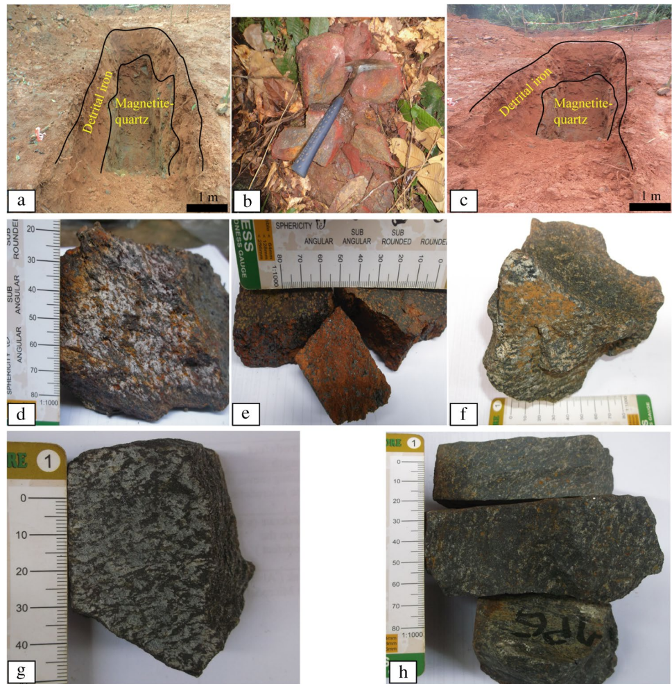
Fig. 5 Field photographs of Kopongo iron ore types: (a) and (c) Detrital iron mineralization. (d) and (e) Quartz-hematite breccia mineralization. (a), (b) and (c) Magnetite-quartz mineralization. (f) and (g) Magnetite mineralization. (h) Enriched magnetite mineralization
