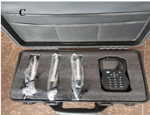
Fig. 2. Field equipment; (A) Fast Pilot Boat, (B) GPS, (C) Multi-parameter water quality analyzer, (D) sample collection bottles.
