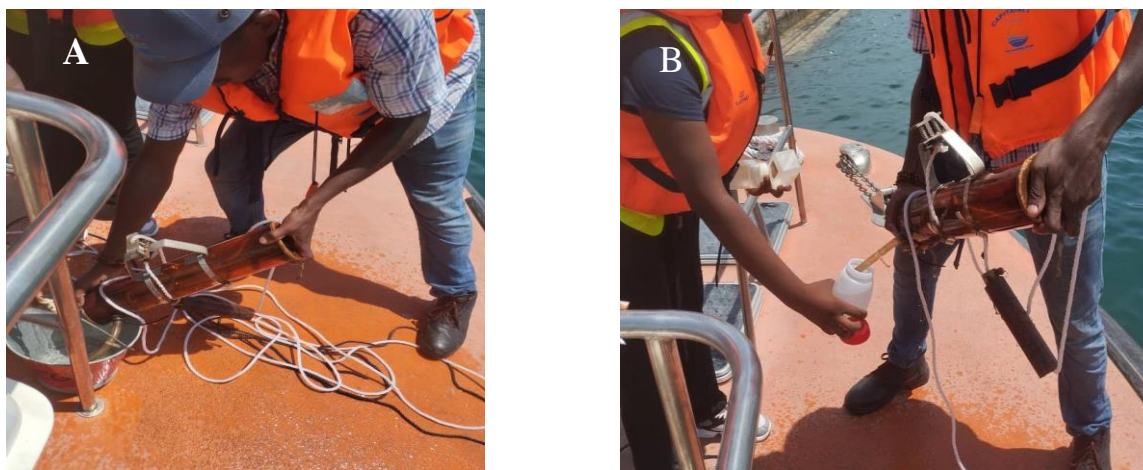
Fig. 4. (A) Water sampling; (B) pouring water sample into a 250ml plastic bottle
