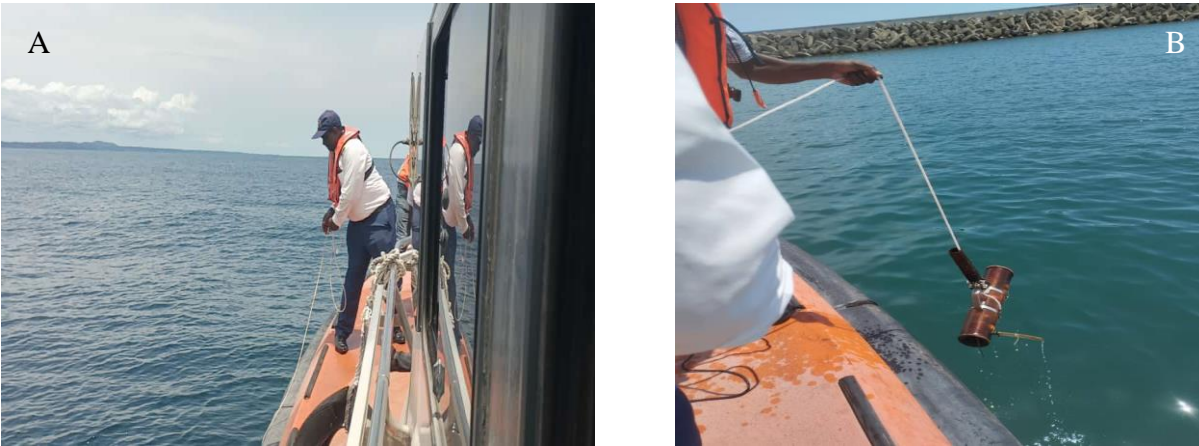
Fig. 5. (A) Seawater collection from the surface; (B) Seawater collection from a depth of 10m below using Van Dorn bottle
