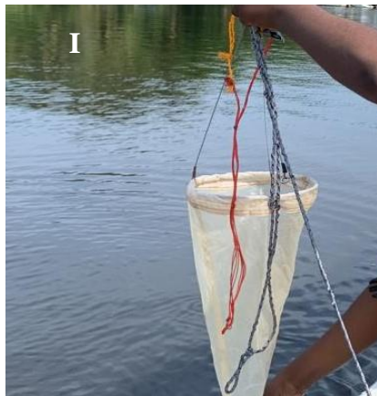
Fig. 3. Collecting equipment; (E) Van Dorn Water Sampler, (F) 250ml sampling bottles in cooler, (G) Lugol solution, (H) BOD bottle, (I) phytoplankton net, and (J) light microscope.
