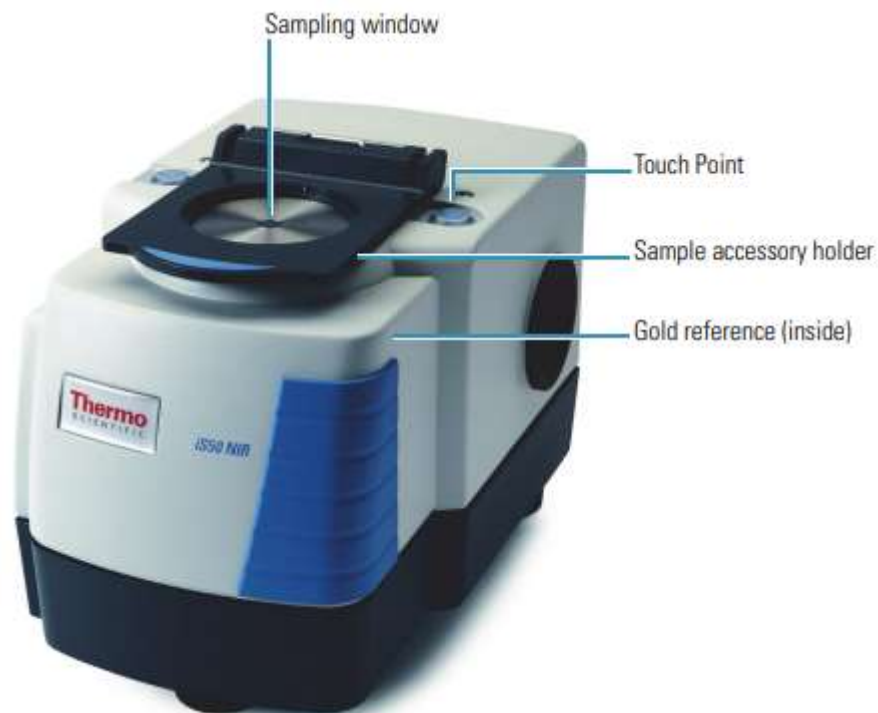
Figure 11: The iS50 NIR Integrating sphere sampling area and features
