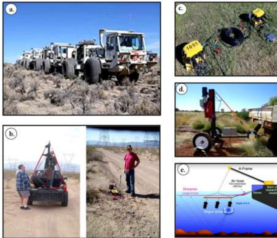
Figure 17. Examples of seismic acquisition sources a) Vibroseis in a set b) Weight dropping and sledge hammer c) geophones d) weight dropping e) Air gun used for marine survey
