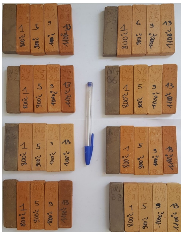
Fig. 8 Visual aspects of fired products of site 1
