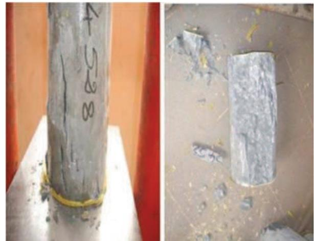
Figure 4. Samples after compressive strength test.
