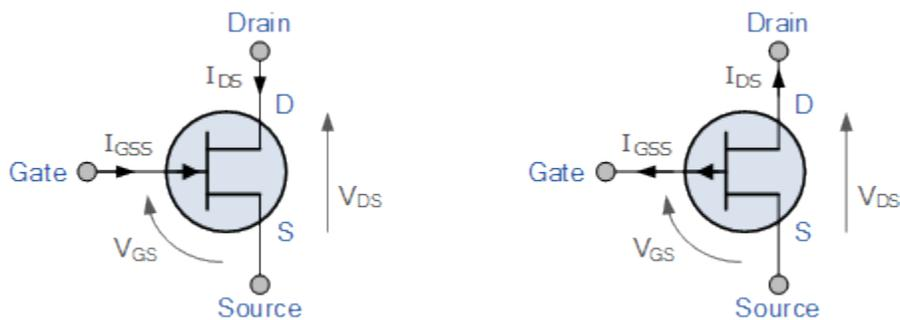
Figure 1.9: a) N-channel JFET; b) P-channel JFET [183]
