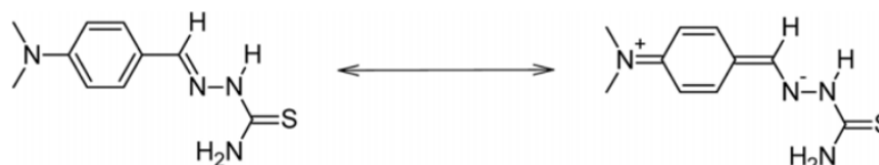
Scheme 2. Resonance structures of thiosemicarbazone moiety (Sampath et al. , 2010).
