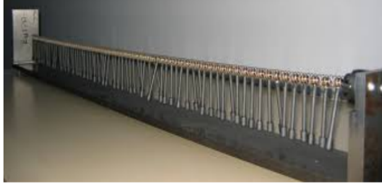
Figure 1.1: Experimental representation of a chain of coupled pendulums [74].
