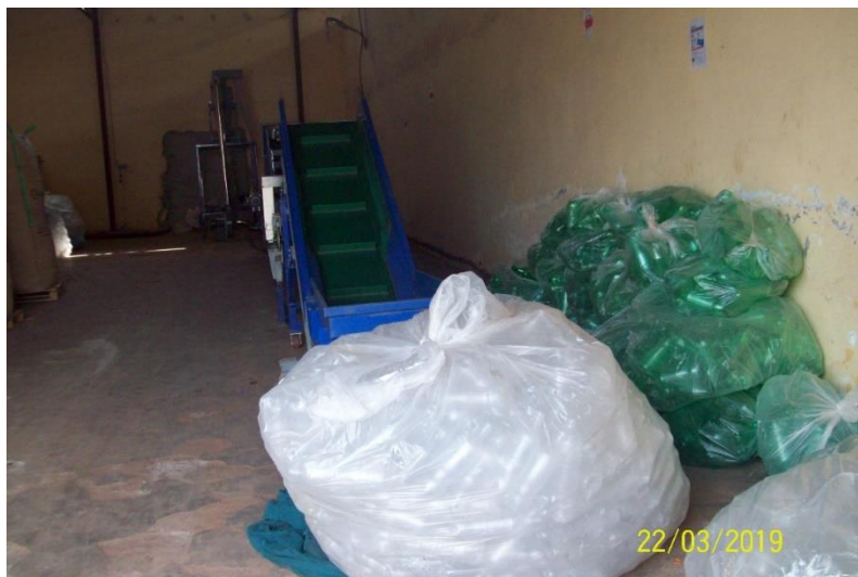
Photo 62: Plastics packaged in front of a vertical axis shredder (Jon Vogler) ready for shredding after sorting and washing in Namé Recycling.
