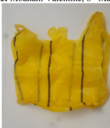
Photo 75: A 12 \mu plastic bag called a two-strip-bag LDPE Black and Yellow colours (32cmx27cm) Source: Mbanam Valentine, 8 th May 2020
