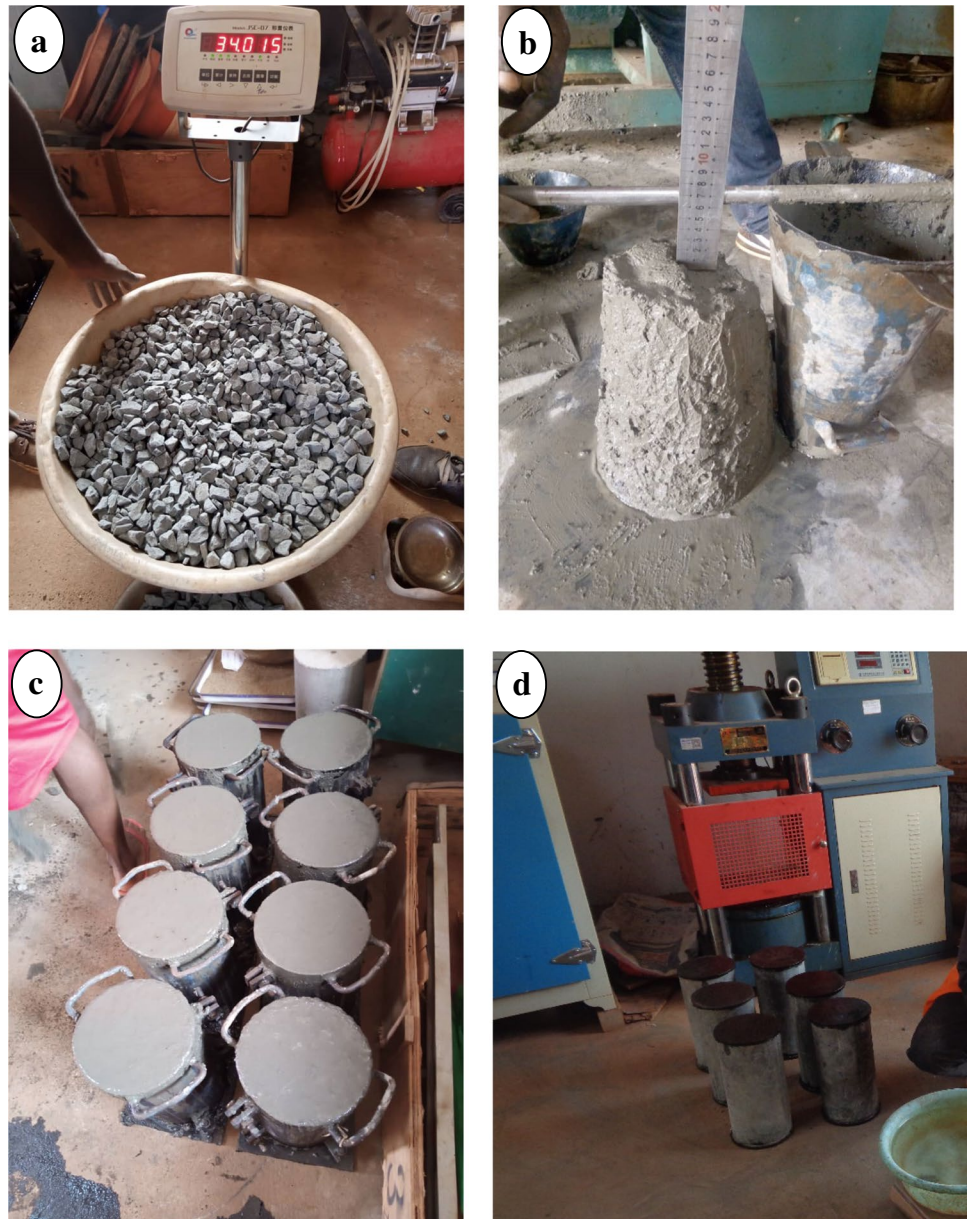
Fig. 2. Sample preparation: a weighing of aggregates; b slump test; c manufactured concrete specimens; d Surfaced specimens for uniaxial compressive strength test
