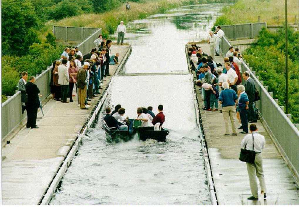
Figure 1.12: Recreation of a solitary wave on the Scott Russell Aqueduct on the Union Canal. Photograph courtesy of Heriot-Watt University [50].
