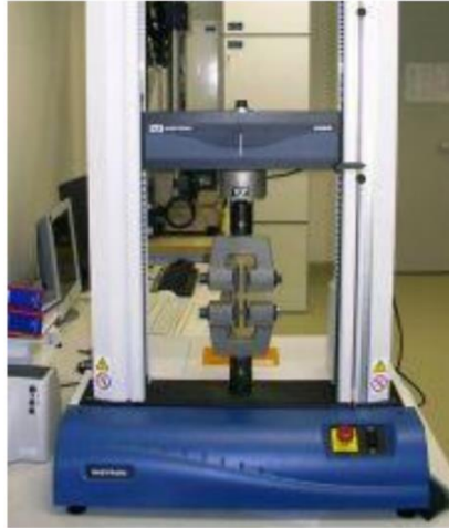
Figure 2.5 Universal machine for mechanical testing
