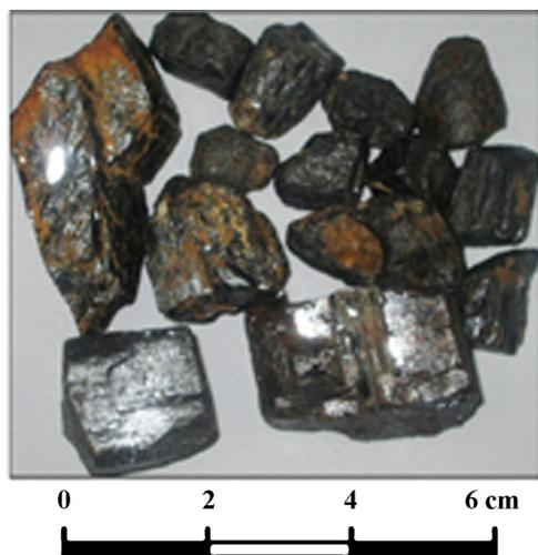
Fig. 3. Rutile grains from the mineralized zone (sandy layer) of the P<sub>2</sub> pit.
