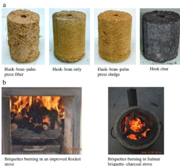
Fig. 2. (a) Different types of briquettes produced from husk-bran mixtures from Engelberg type mills and rice husk char; (b) burning of rice-husk briquettes in rocket and Salmar briquette-charcoal stoves.
