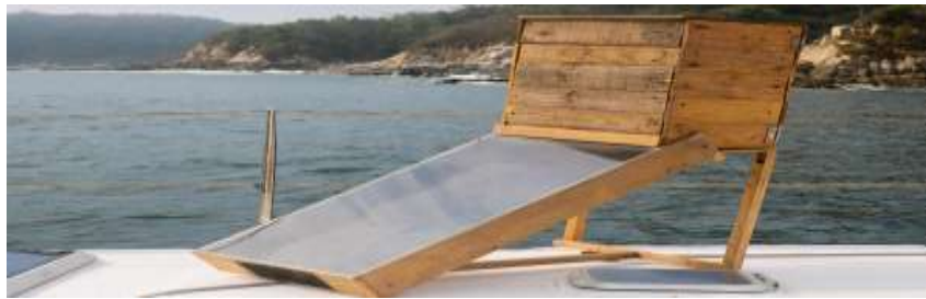
Photo 10: Séchoir solaire indirect
