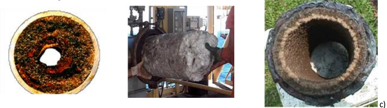
Figure 1.1: some flow assurance issues deposition inside pipeline [6]. In a) wax deposition, b) hydrate deposition and c) asphaltenes deposition.
