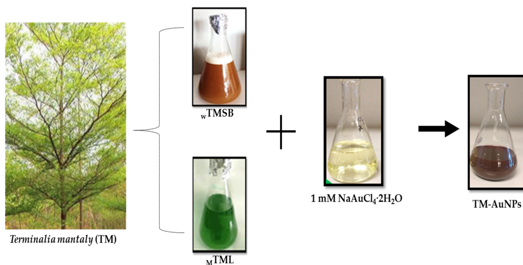
Figure 1. One step synthesis of TM-gold nanoparticles (AuNPs) by the reduction of chloroaurate ions by TM extracts. The w TM and M TM extracts of leaf, root and stem/bark parts of the plant were prepared and mixed with \text{NaAuCl}_4 \cdot 2\text{H}_2\text{O} . The appearance of a red wine/ruby red color indicated the formation of the AuNPs.
