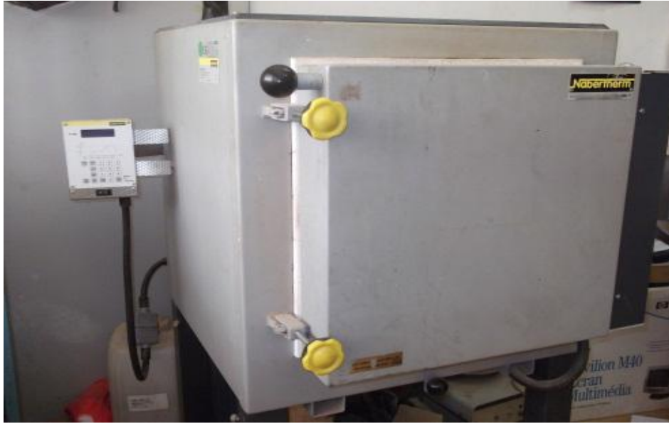
Figure 6: Electrical furnace (Nabertherm, model LH 60/14) used.
