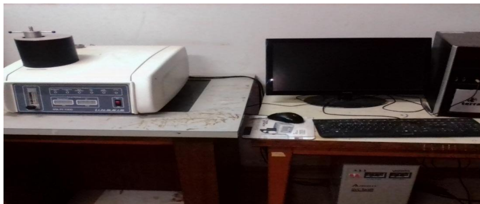
Figure 8: Thermal analysis device (LINSEIS STAPT-1000) used.
