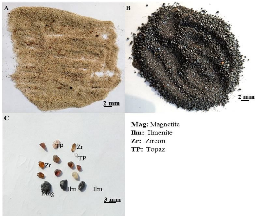
Figure 66: Pan concentrate from Mayo Kila. A: non-magnetic minerals, B: Magnetic minerals and C: Magnetic and non-magnetic minerals.
