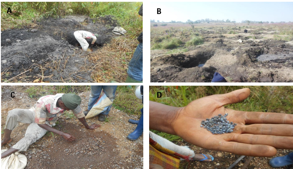
Figure 17: Sapphire exploitation in Mbiame along the Mbven Placer. A: Pitting and water removal from pit, B: abandoned pits, C: Hand picking of sapphire, D: panned sapphire grains
