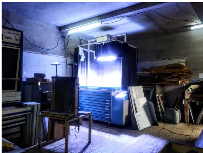
Insoleuse during insolation
