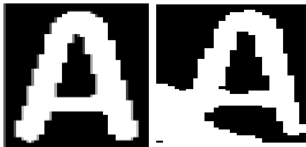
Figure 1: Examples letter "A" printed with laser radiation stable (left) and unstable laser radiation (right) [23].
