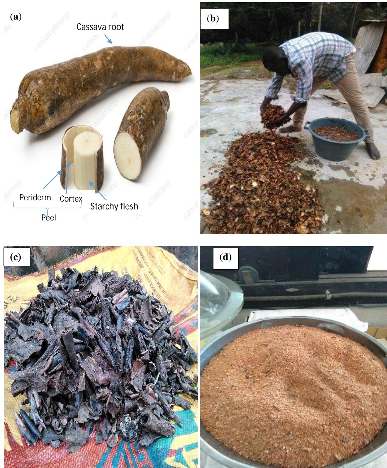
Figure 5: (a) Whole cassava root and peeled pieces; (b) Washing and drying of cassava peels; (c) Cracked cassava peels and (d) Cassava peel ash used.
