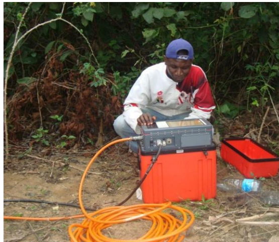
Photo 1 : Recording of AMT data in a remote area (Profile 1).
