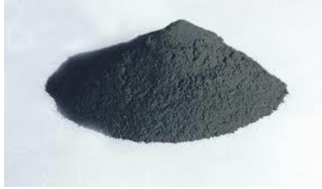
Figure 7: Powder activated carbon
