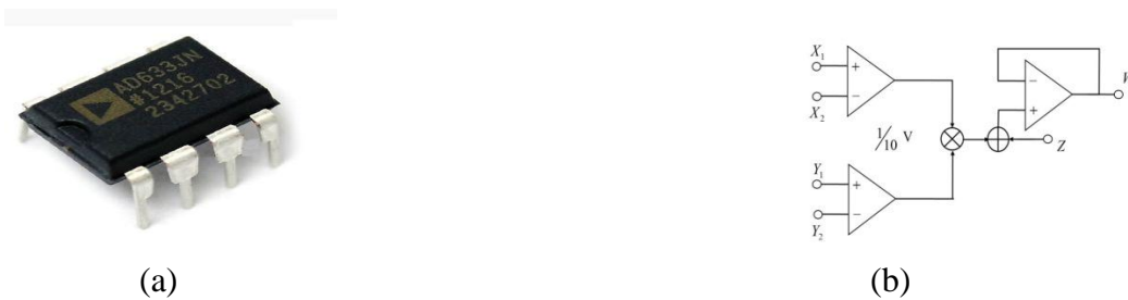
Figure 2.2: (a) Example of analog multiplier AD633JN and (b) electrical equivalent of the analog multiplier.
