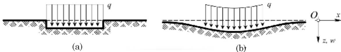
Figure 1.11: Deflections of elastic foundations under uniform pressure: (a) Winkler foundation; (b) practical soil foundation
